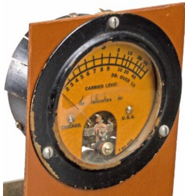
Anode current meter in the push-pull RF amplifier. This meter was originally a 'S' meter from an American Hallicrafters Model S-36A communications receiver. AWM PAIU2011_165_38
